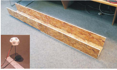
FIG. 8. (Color online) Photograph of the long room tenth scale-model with the top and two ends open. Bottom left shows the miniature dodecahedron loudspeaker.
